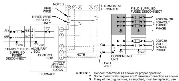
Fig. 8—Heating and Cooling Application Wiring Diagram
